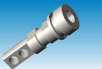
**TERMINAL CONSTRUCTION** - The contact quality between the insert terminal and the lead post is of vital importance during short duration / high Amp discharges. Elevated terminal temperatures are the result of poor contact, eventually causing seal degradation and electrolyte leaks. Haze design and assembly technique for terminal casting ensures trouble free operation for the design life of the battery.
